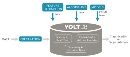
The diagram above illustrates an example architecture that shows essential machine learning modules (including feature extraction), algorithms and trained models that are built on separate platforms, and then are ingested and deployed in VoltDB through java and PMML.
